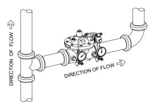
TYPICAL INSTALLATION (MODEL ZW209FP with gauge 2005-25UL)
