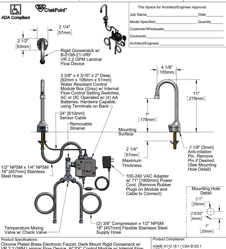
Chrome Plated Brass Electronic Faucet: Deck Mount Rigid Gooseneck w/ VR 2.2 GPM Laminar Flow Device, AC/DC Control Module w/ Internal Flow Control Setting Switches, Temperature Control Mixing Valve w/ Check Valves, 18" Flexible Stainless Steel Supply Hoses
