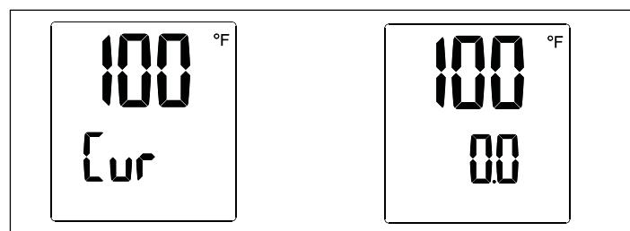
The accumulated cost savings updates daily, and shows the estimated savings for the user compared to an installation where a 50-gallon tank-type water heater was used.
