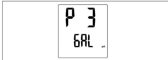
The current volume unit will be displayed and the value will be flashing to indicate that it can be changed. Rotate the control knob to change the value between gallons per minute and liters per minute.
