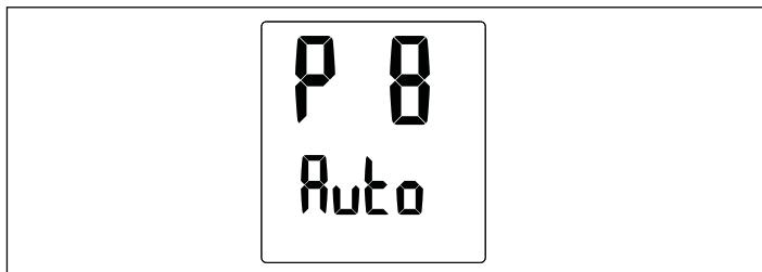
The entire display and backlight will be flashing to indicate that the value can be changed by rotating the control knob. When the value is set to "On", the backlight will always be on. When the value is set to "Auto", it will automatically deactivate after 30 seconds of inactivity.
