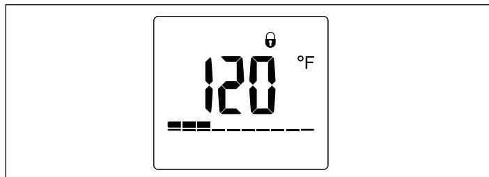
If the display-lock is active, a lock symbol will appear on the base display, and no parameters can be changed. In order to disable the lock, hold the T<sub>max</sub> button for 12 seconds. The lock will disappear from the display and all parameters can be changed again.
