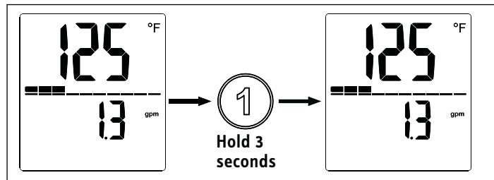
To change the value of either preset 1 or preset 2, first rotate the control knob to the temperature that you want to set as the preset value. Then hold the preset button for 3 seconds. The display will flash to indicate that the preset has been changed successfully.
