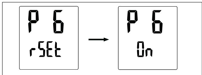
The display will be flashing to indicate that the value can be changed by rotating the control knob. To reset, first press and hold both buttons 1 and 2 for 5 seconds, "On" then appears. Then push information button for 5 seconds to reset.
