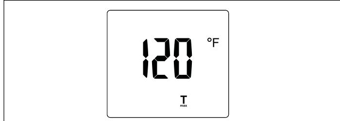
At the  $T_{max}$  setting menu, the display will flash, indicating that the value can be changed by rotating the control knob. The  $T_{max}$  value can be increased by turning the control knob clockwise, and decreased by turning it counter-clockwise. The  $T_{max}$  value can be deactivated by turning the control knob counter-clockwise, past the 68 °F (20 °C) setting. The display will read "Off" if  $T_{max}$  is inactive.
