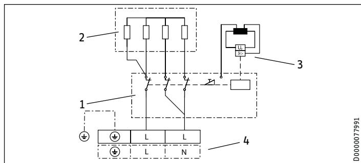
1 Power PCB with integral safety switch
