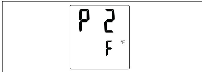
The current unit will be shown and the secondary display value will be flashing to indicate that the value can be changed. Rotate the control knob to change the value between degrees Fahrenheit and degrees Celsius.
