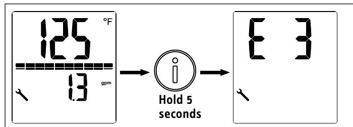
While the wrench is showing, press and hold the Information button (DHC-E Plus) or Tmax button (DHC-E Trend) for five seconds to advance the display to the error display page. Consult section 16, "Troubleshooting", pg. 22, for information on how to interpret the reported error code.
