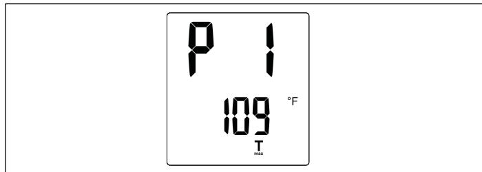
At the T<sub>max</sub> setting menu, the temperature value will flash, indicating that the value can be changed by rotating the control knob. The T<sub>max</sub> value can be increased by turning the control knob clockwise, and decreased by turning it counter-clockwise. The T<sub>max</sub> value can be deactivated by turning the control knob counter-clockwise, past the 68°F (20°C) setting. The display will read "Off" if T<sub>max</sub> is inactive.
