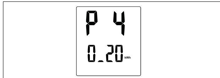
The secondary display will be flashing to indicate that the value can be changed by rotating the control knob. Consult your electricity bill to determine the cost of electricity per kWh.
