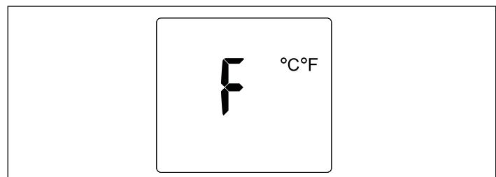
The current unit will be shown and the display will be flashing to indicate that the value can be changed. Rotate the control knob to change the value between Fahrenheit and Celsius.
