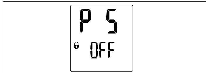
If the display-lock parameter is set to "On" and the user either holds the Information button for 5 seconds or lets the display time out for 15 seconds, the display-lock will become active.
