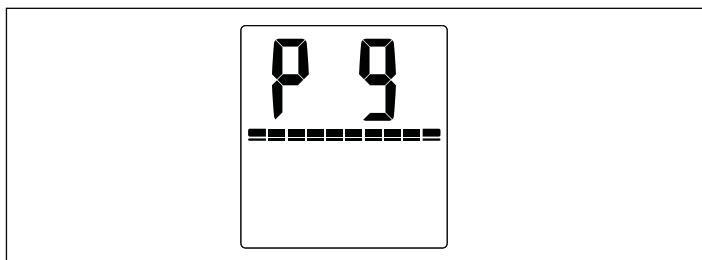
The power capacity status bar indicates the brightness setting. A full capacity bar indicates that the brightness is at the high setting. Two capacity bars indicate that the brightness is at the low setting.
