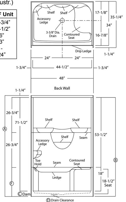
**Illustrations 1a - Center Drain, Unit Dimension & Alcove Framing Guidelines (dimensional tolerance +0 / -3/8")**
