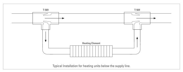
These diagrams are representative of typical installations. It is recommended that flowrate and pressure loss requirements are calculated for the specific system in which the mono-flow or venturi tee(s) are being installed. The manufacturer of the heating element should provide performance parameters associated with various flow rates.
