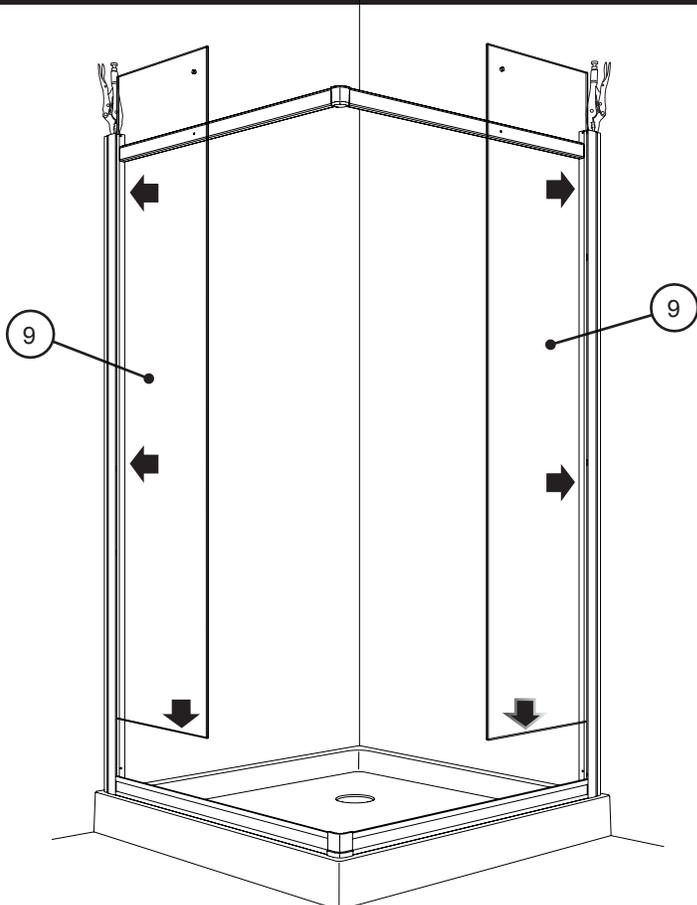
**13** **INSTALL THE GLASS FASTENERS / INSTALLER LES FIXATIONS DE VERRE**
