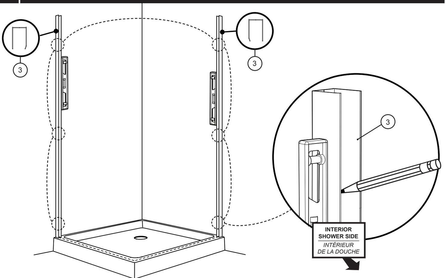
**5** DRILL, APPLY SILICONE AND INSERT WALL PLUGS
