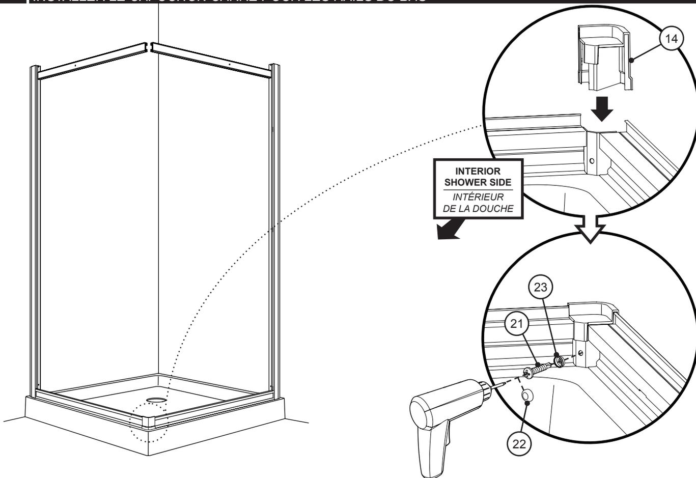
**9 ASSEMBLE THE TOP FRAMES TOGETHER WITH RAIL FASTENER**
