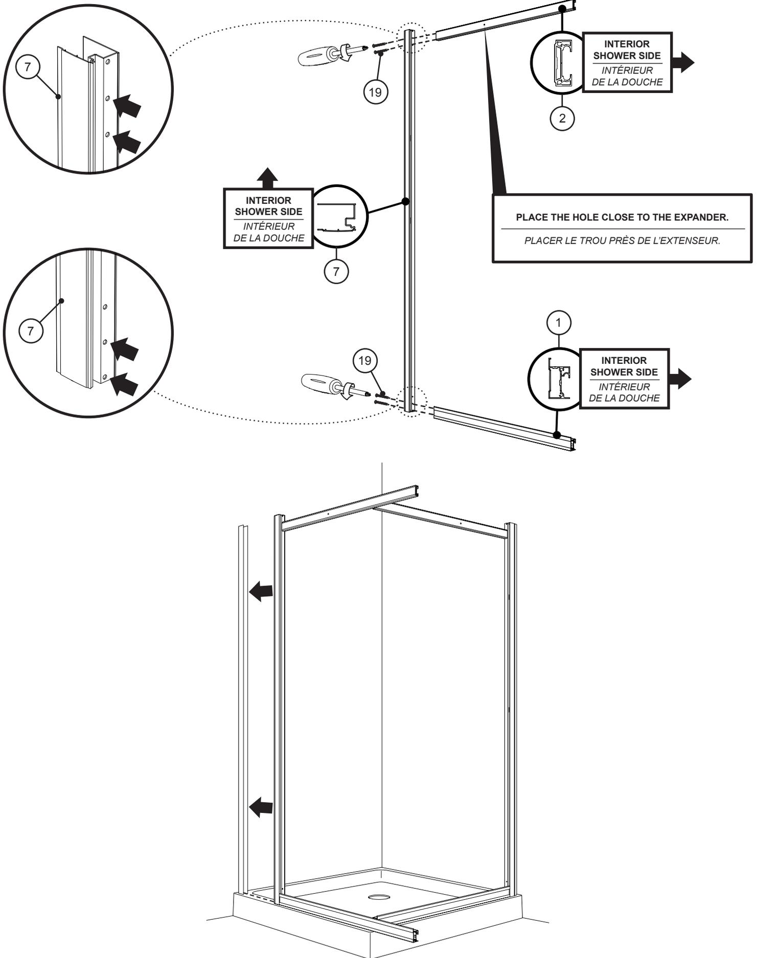
**7 ASSEMBLE THE BOTTOM FRAMES TOGETHER WITH RAIL FASTENER**
