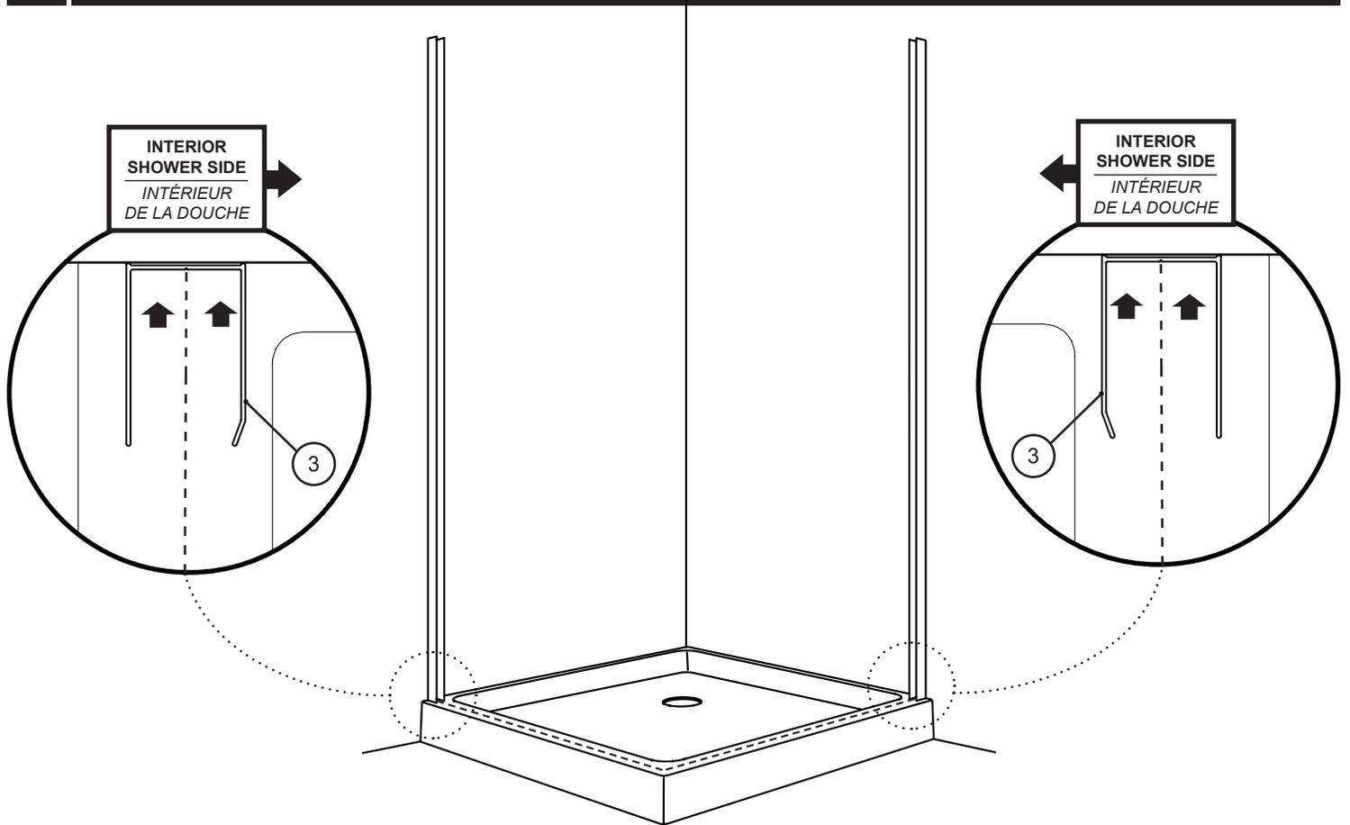
**4 MARK THE DRILLING LOCATIONS / MARQUER LES POINTS DE PERÇAGE**
