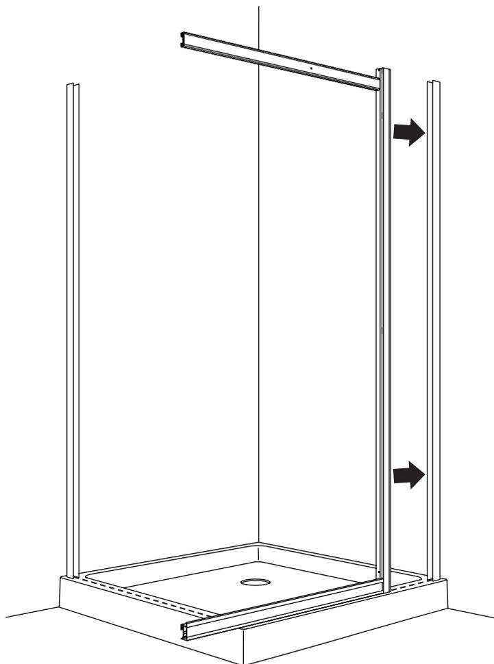
**8 ASSEMBLE THE OTHER SIDE OF THE FRAME AND INSERT INTO THE WALL JAMB**
