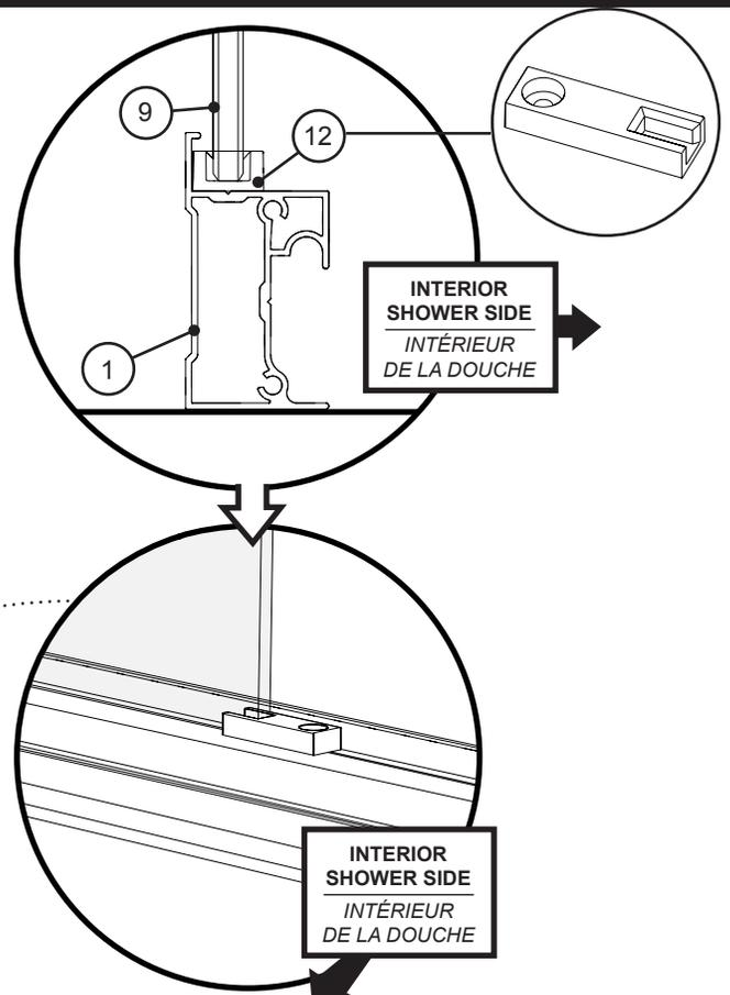
**15 SECURE THE BOTTOM SUPPORTS / SÉCURISER LES SUPPORTS DU BAS**
