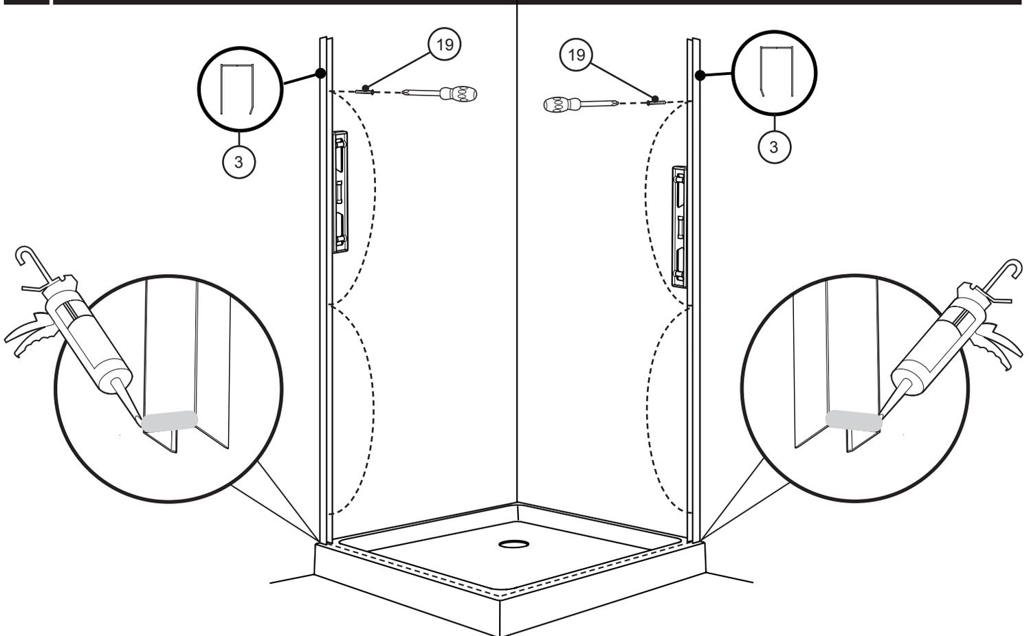
**7 ASSEMBLE ONE SIDE OF THE FRAME AND INSERT INTO THE WALL JAMB**
