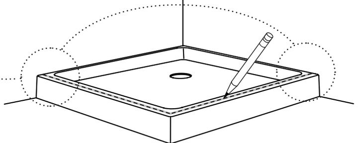
**3 PLACE CENTER OF WALL JAMB ON THE LINE / PLACER LE CENTRE DU JAMBAGE SUR LA LIGNE**
